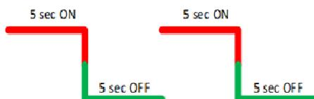
**LNG LEAKAGE ALARM**
